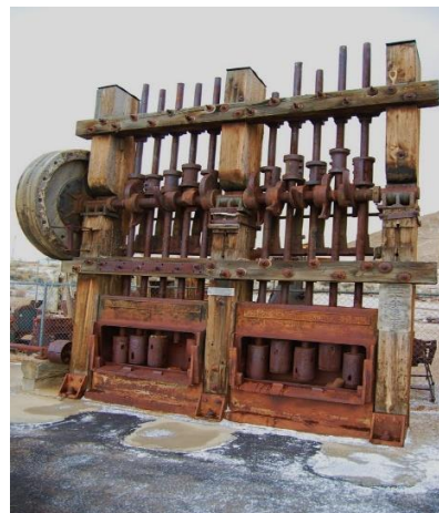
Ten stamp mill battery mill (Courtesy of Central Nevada Museum)
